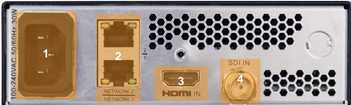
Figure 2: Impulse 300E Rear Panel
