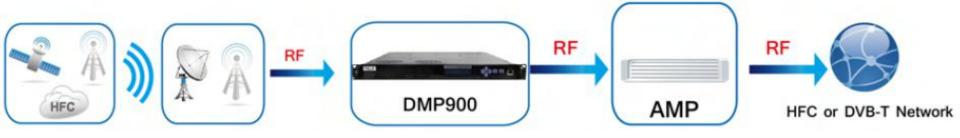
With receiver, QAM or OFDM module in chassis, 1 DMP can transmodulate up to 16 DVB-S2/T/T2 channels to QAM or OFDM signal directly. It's especially suitable for HITS, hotel, community and other SMATV.
